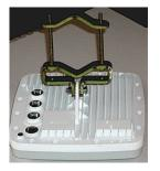
3. Place the radio with mounting bracket at the desired height on the pole and slide the top part of the bracket onto the mounting screws. Screw on the nuts and firmly tighten.
